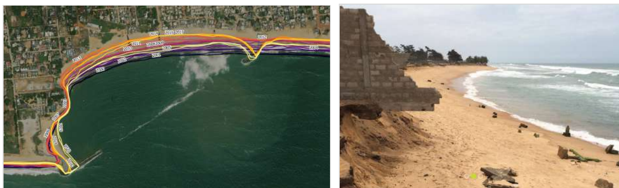
Changes in coastline positions due to erosion and deposition around marine infrastructure, Cotonou, Benin, 2000–2017 (Digital Earth Africa).
